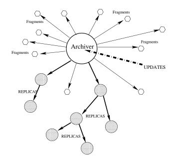
**Fig. 1.** Hybrid Update Architecture: Updates are sent to a central "Archiver", which produces archival fragments at the same time that it updates live replicas. Clients can achieve low-latency read access by utilizing replicas directly.
